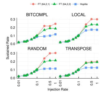
Figure 11: Effect of various 64 PE FastTrack NoCs (D,R) combinations) on sustained rate for synthetic traffic.
