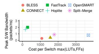
Figure 1: Area-Bandwidth Tradeoffs in implementing NoCs on FPGAs.
