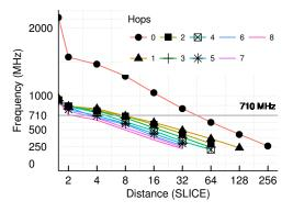
Figure 6: Quantifying the impact of express physical bypass channels on frequency of the resulting design.
