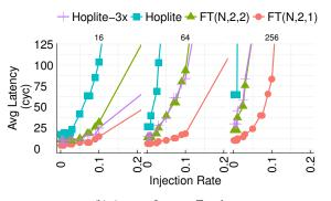
(b) Average Latency Trends Figure 13: Measuring the effect of multiple physical channels on Hoplite vs. FastTrack for N=16, 64, and 256.
