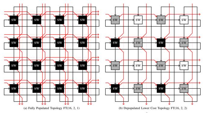
Figure 7: FastTrack Topology for a  $4 \times 4$  Torus NoC with D=2. The notation is FT ( $N^2$ , D, R). The red wires represent express links that exploit faster FPGA routing resources to bypass multiple NoC routers. Wraparound links are shown with dotted lines. The shades correspond to FastTrack router complexity, with darker switches being more expensive.
