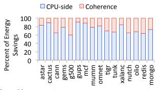
Figure 11: Percent of the energy savings that can be attributed to savings in CPU-side lookups versus coherence lookups. Results are collected on an out-of-order system with 64KB L1 caches at 1.33GHz.
