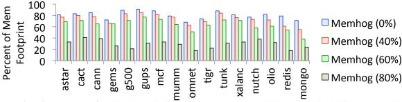
Figure 3: Fraction of total memory footprint allocated with 2MB superpages on a real 32-core Intel Sandybridge system with 32GB of memory. We show how superpage allocation varies as memory is fragmented with the memhog workload.
