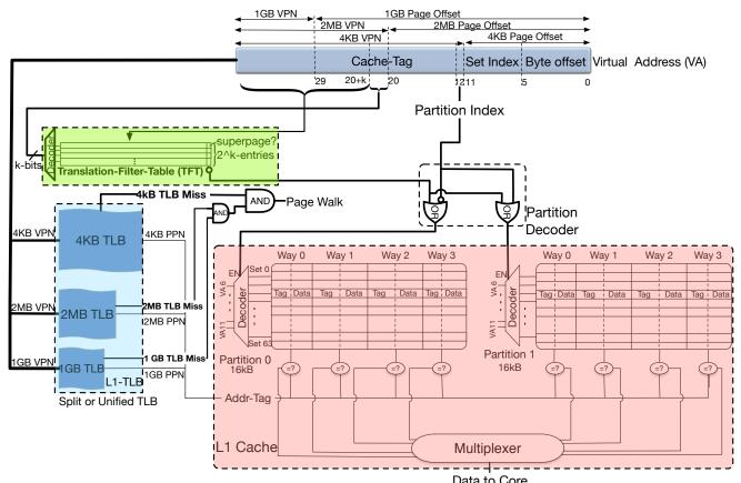
Data to Core Figure 4: SEESAW for a 32KB data cache. SEESAW is amenable to both split TLB and unified TLB configurations.
