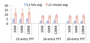
Figure 13: Percentage of superpage accesses that are missed by the TFT, for varying TFT size (12- to 20-entry) and cache size (32KB, 64KB, 128KB). Results are separated for TFT misses for accesses that hit and miss in the data cache. Average, min, and max results shown.
