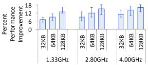
Figure 9: Runtime improvement using SEESAW on an in-order processor versus baseline VIPT. We show the average, minimum, and maximum improvements across all workloads for all cache sizes, across 1.33GHz, 2.80GHz, and 4.00GHz operating frequency. Benefits are higher on an in-order versus out-of-order processor.
