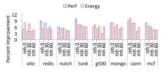
Figure 12: We vary memory fragmentation using memhog, which uses 0%, 30%, and 60% of memory. We show percent performance and energy savings on the memory hierarchy by using SEESAW.
