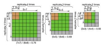
Figure 6: The overall utilization rate of selecting  $T\_R = T\_Y = 2$  when *R* and *S* are both equal to 7, 5, 3 respectively. Green area shows the filter weights and the brown area in the upper-left shows a tile. The gray area around the green area shows invalid coverage of tiles, which is out-of-bound that causes significant underutilization as presented at the bottom of each example.
