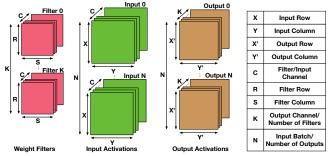
Figure 4: Loop variable convention for a convolutional layer.
